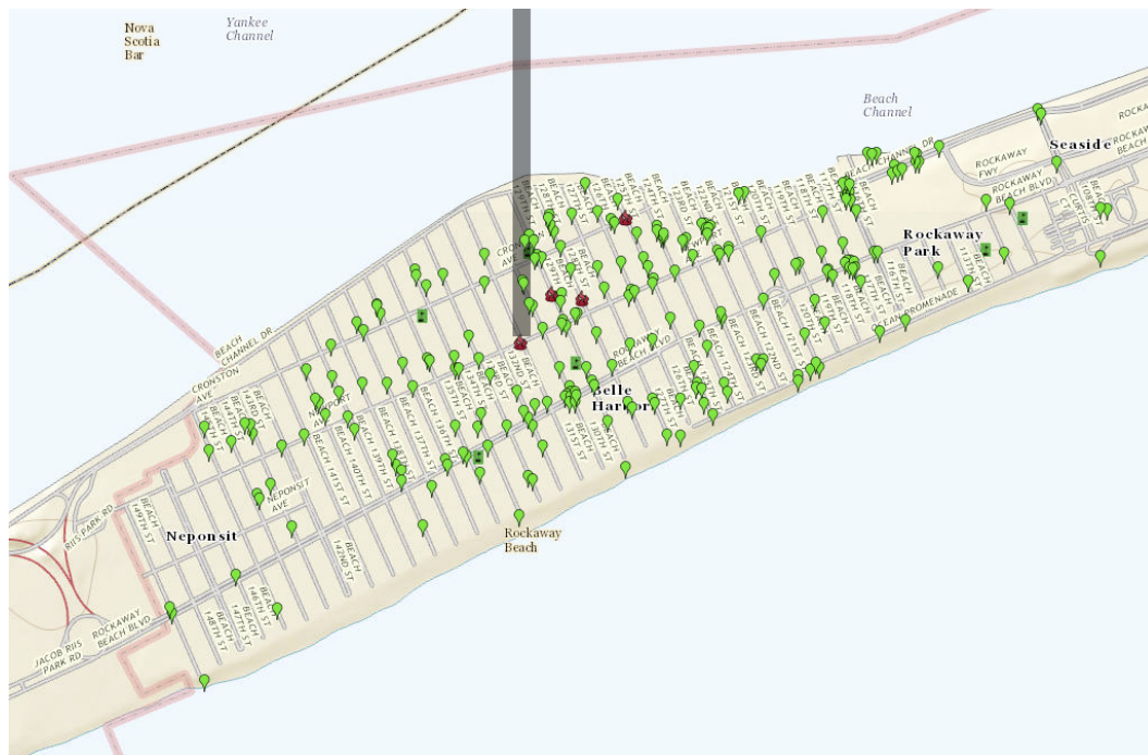
Figure 2. Belle Harbor Eyewitness Locations. The gray line ending in a red marker shows the path of the main body of the aircraft. Each green marker is an eyewitness, the other red markers show final location of the engines and left wing tip.
