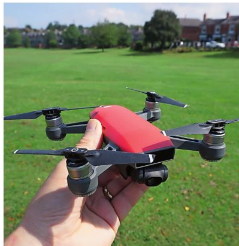
The tiny, 0.3kg (11oz) DJI Spark is replacing larger drones like the Phantom. Operator's hand lends scale
