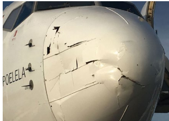
This damage to an airliner in Mozambique was at first blamed on a drone, but it resulted from structural failure.
